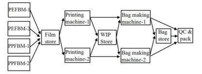
Figure 3. Network diagram of manufacturing system. PEFBM and PPFBM indicate Polyethylene Film Blowing Machine and Polypropylene Film Blowing Machine, respectively.
