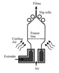
Figure 1. Simplified film blowing process.
