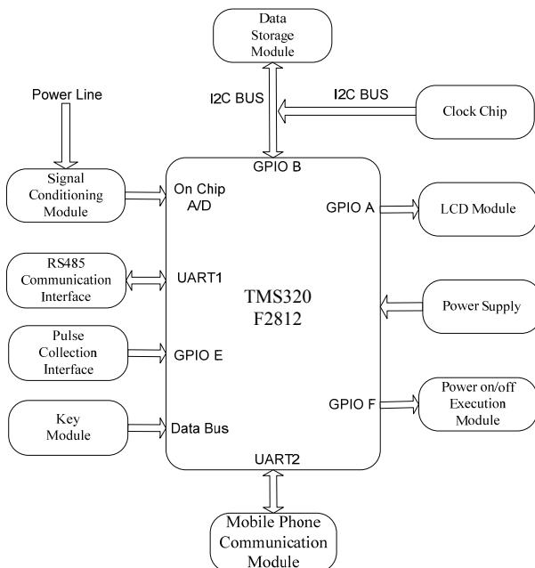
**Figure 1. Hardware block diagram.**
