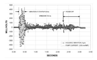
Figure 3. Pump vibration and motor current at start-up and shut-down of a Cleveland Heart VAD.
