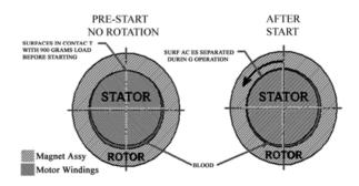
**Figure 2.** Journal bearing. Left: Inner surfaces of the RA are in contact with stator when pump is not running. Right: After starting, the RA is separated from the stator and rides on a film of blood during operation. Assy, Assembly.
