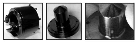
Figure 4. BMF-coated RVAD RA (left) and stator assembly (middle); commercial DLC-coated stator assembly scratches post-test (right).
