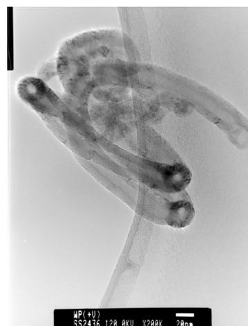
**Figure 3. TEM micrographs of CNT (obtained by pyrolyzing HDPE in hydrogen atmosphere for 2 h at  $1050^\circ\text{C}$  showing coiled multi walled carbon nano tubes.**
