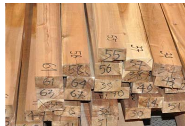
Figure 1. Akasia wood used as shear wall frames member.
