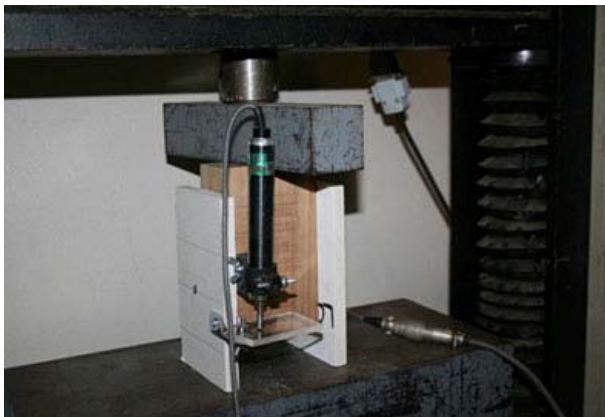
Figure 7. Shear test specimen of Akasia wood and FCB fastened by N75 nail during test.
