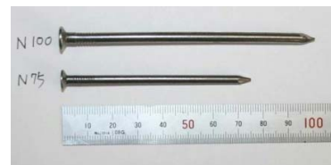
Figure 3. The steel nail used as fastener for all connection.
