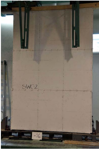
Figure 10. The C brace with CFB sheathed during test.
