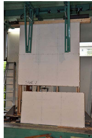
Figure 23. The specimen at final condition in 1/15 radian-deformation level.
