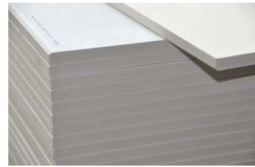
Figure 2. FCB used as frame specimen sheathed.
