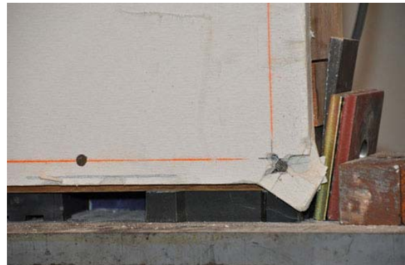
Figure 22. Initial failure at edge nail in 1/75 radian deformation level.
