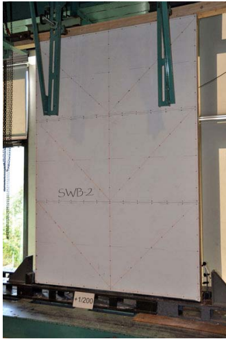
Figure 9. The V brace frame CFB sheathed during test.
