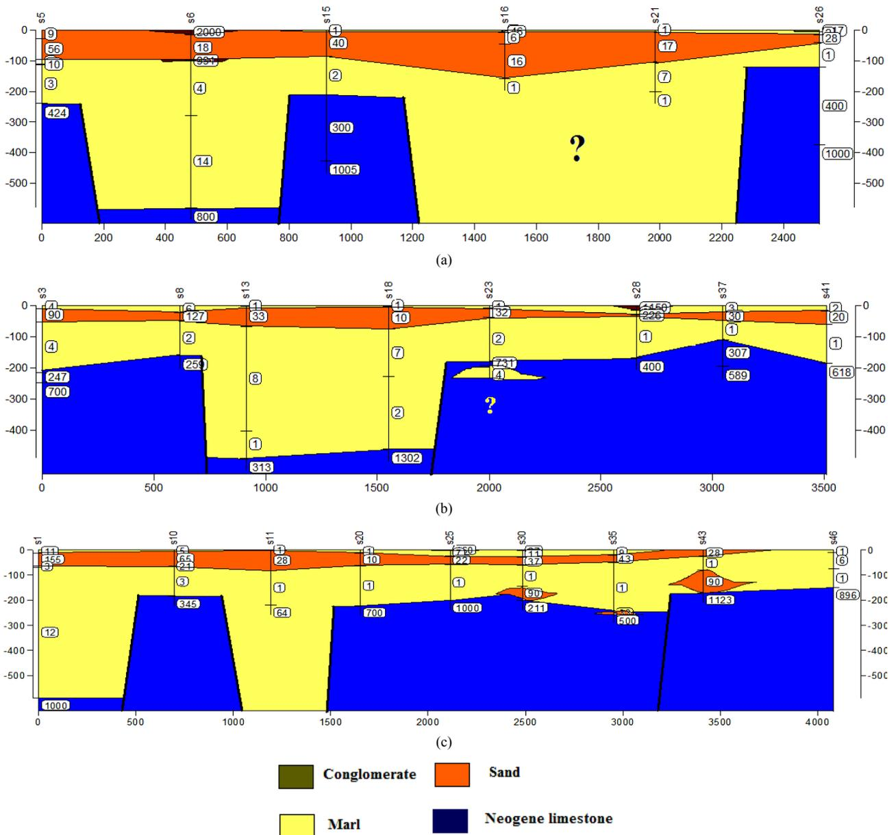
Figure 5. North West-South East geoelectric sections, perpendicular to Draa Outita ridge.
