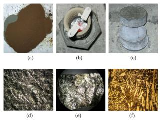
Figure 4. Restoring metals and obtaining complex alloys from powder oxide industrial waste via the SHS method. (a) Reactive mixture of powder industrial waste of manganese and silicium rust with metal aluminum; (b) SHS processing of waste; (c) Obtained metal alloy and slag of restoration process (Korund, Spinel); (d) Surface of metal alloy ( $\times$ 50); (e) breaking-off of metal alloy ( $\times$ 10); (f) Microstructure of metal alloy ( $\times$ 100).
