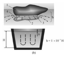
Figure 5. Activization of metallothermic SHS briquettes in liquid steel. (a) Self-recovery of metals (Mn-V), ×50; (b) Schematic model; 1—Oxidic phase of reducing alloying element; 2—Reducer (aluminium); 3—Zone of exothermic reaction in the briquette; 4—Drops of reduced metallic element; h—Zone of reduction and deposition of alloying element from briquettes to ladles; H—Filling level of ladle by treating liquid steel.
