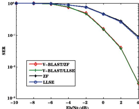
**Figure 2.** Symbol error rates (SER) of VBLAST/ZF, VBLAST/LLSE, ZF and LLSE receiver.
