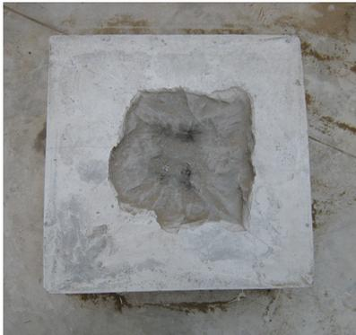
Figure 6 Test block explosion
