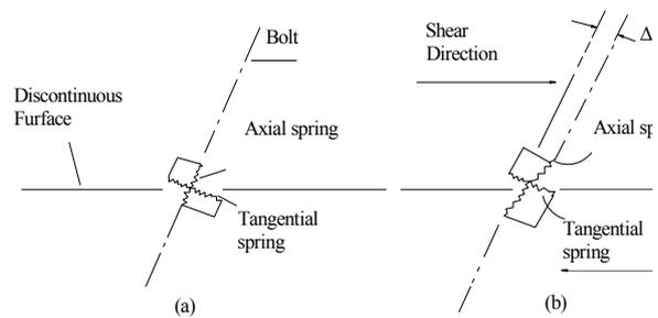
**Fig.2 The anchor-injected bolt contrast figure in forward (a) and rear (b)**
