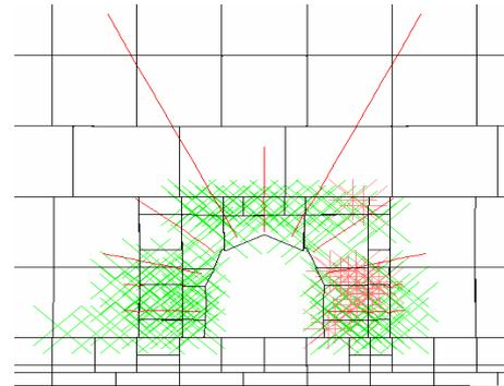
(b) Enlarged drawing under bolting anchor-injected support
