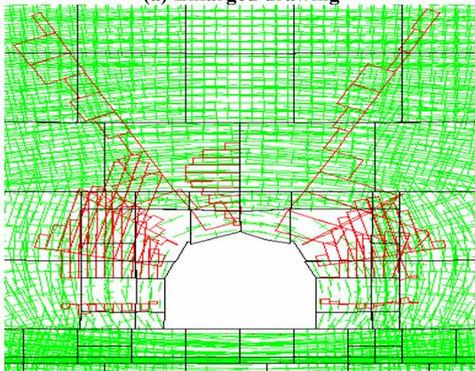
(b) Enlarged drawing under bolting anchor-injected support
