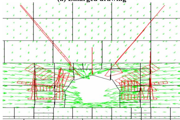
(b) Enlarged drawing under bolting anchor-injected support
