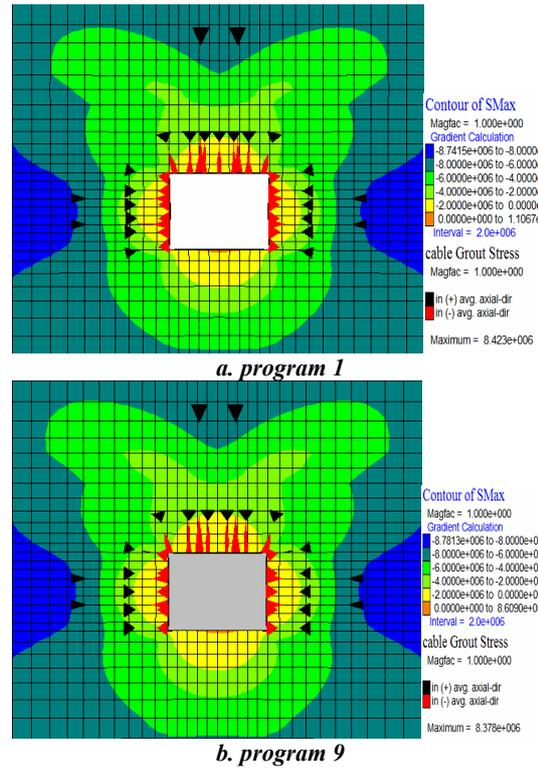
**Figure 3. Comparison of Min-stress distribution**
