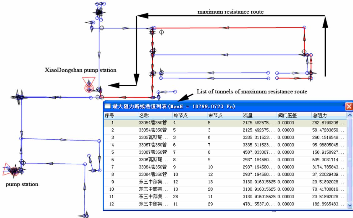
Figure 3. The resistance route diagram of Third East Area after when the XiaoDongshan pump station is built
