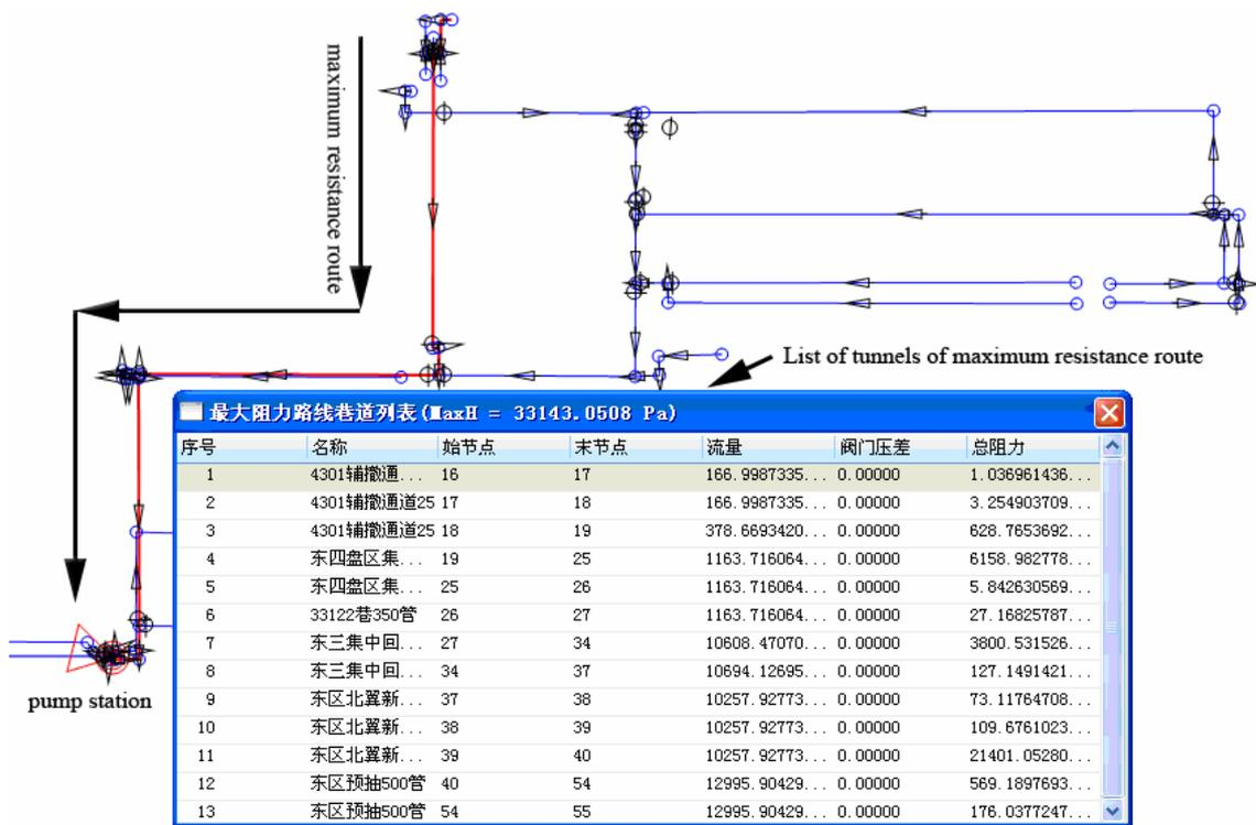
Figure 2. The diagram of maximum resistance route of pumping pipeline system
