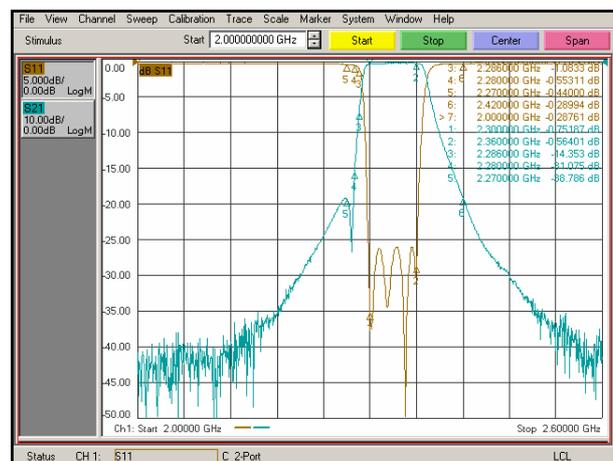
Figure 9. test S parameter curve of filter
