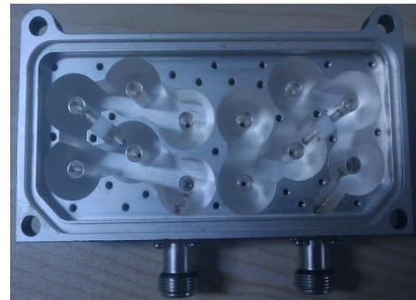
Figure 8. Filter real object (same double filters)
