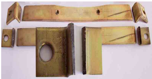
Figure 2b. Prop up to transform and split 图 2b. 支撑架变形和断裂
