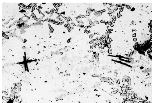
Figure 7 Irony phase in the etallographic structure
