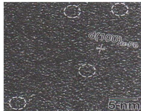
Figure 12. HRTEM pattern of the as-quenched  $Fe_{83.3}Si_4B_8P_4Cu_{0.7}$  ribbon<sup>[8]</sup>
