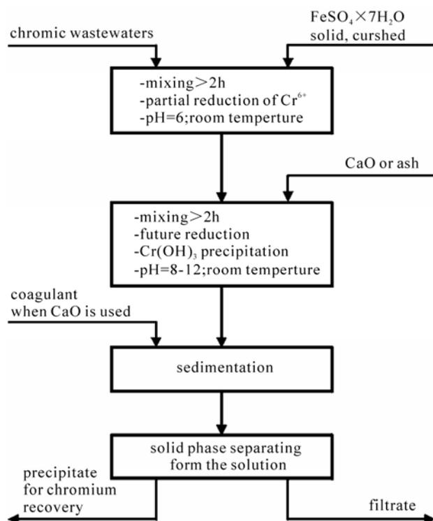
**Figure 4.** Block diagram showing the removal procedure of chromium (VI) from wastewater in the “Alwernia” Chemical Works.
