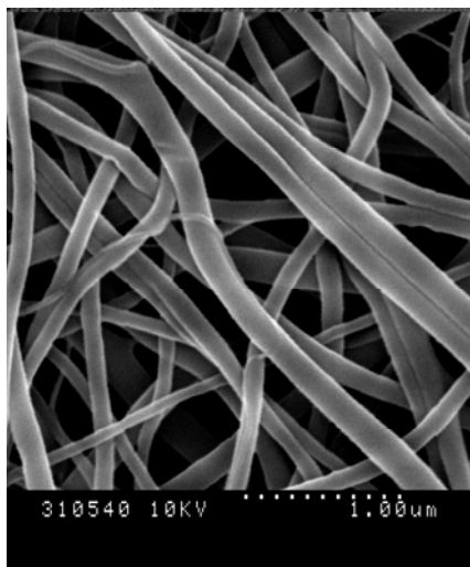
Figure 2. SEM images of 22%(w/w) nylon-6 in formic acid fibers electrospun at 18 kV
