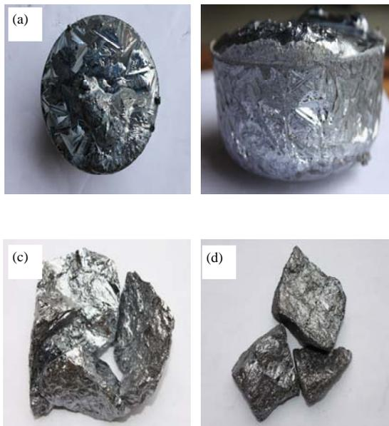
Figure 2. The photos of silicon ingot and the slices of silicon ingot (a) the top surface, (b) the side surface, (c) the silicon ingot after solidification and (d) the raw metallurgical silicon
