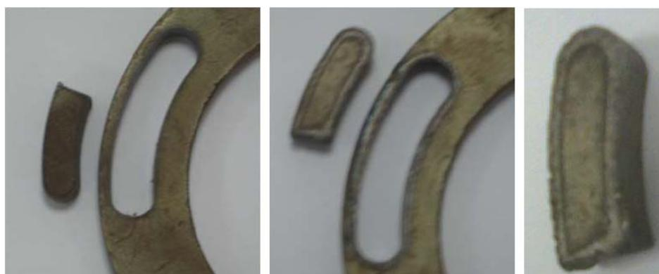
Figure 3 Both sides of 8mm NdFeB specimen after laser cutting
