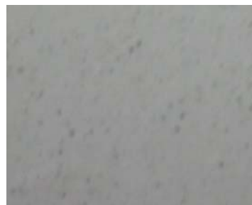
Figure 4. the surface image of coating with nano-ZnO addition 图 4. 添加 nano-ZnO 颗粒后涂层表面情况
