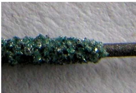
Figure 2 Tungsten Rhenium alloy wire failed
