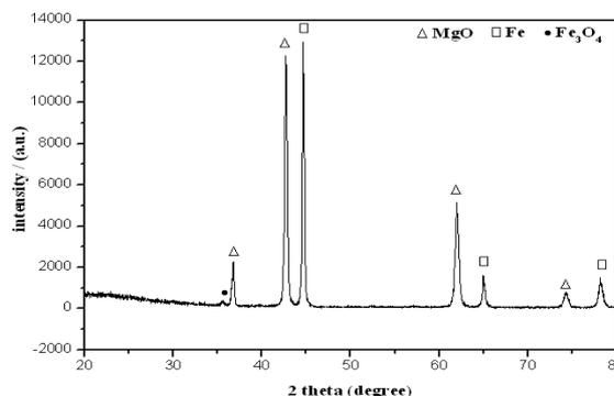
Figure 3. XRD patterns of the sintered samples at  $5^\circ\text{C}/\text{min}$  heating rate
