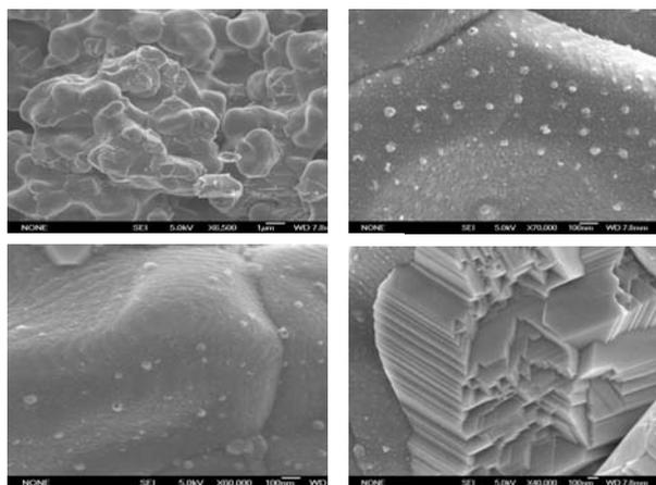
**Figure 6.** SEM micrograph of the Mg-70.9wt%Fe<sub>3</sub>O<sub>4</sub> samples at 8°C/min heating rate
