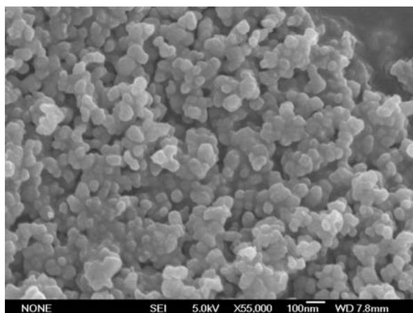
**Figure 5.** SEM micrograph of the Mg-70.9 wt.% Fe<sub>3</sub>O<sub>4</sub> samples at 5°C/min heating rate
