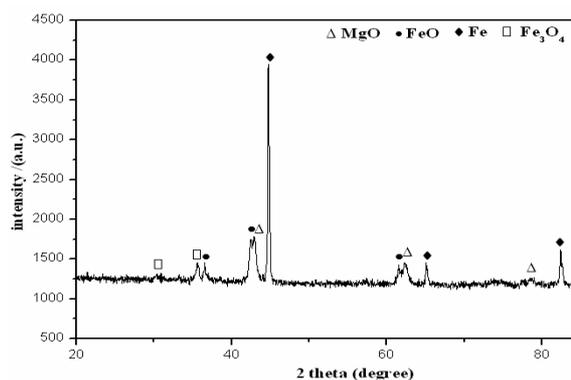
Figure 2. XRD patterns of the sintered samples at  $2^\circ\text{C}/\text{min}$  heating rate
