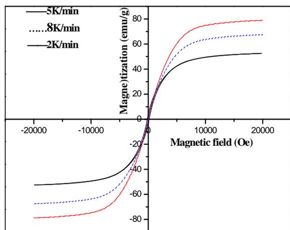
**Figure 7. M-H hysteresis loops of the Mg-70.9 wt.% Fe<sub>3</sub>O<sub>4</sub> samples sintered at different heating rates**
