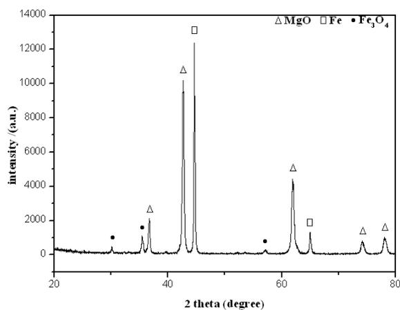
**Figure 4.** XRD patterns of the sintered samples at 8°C/min heating rate
