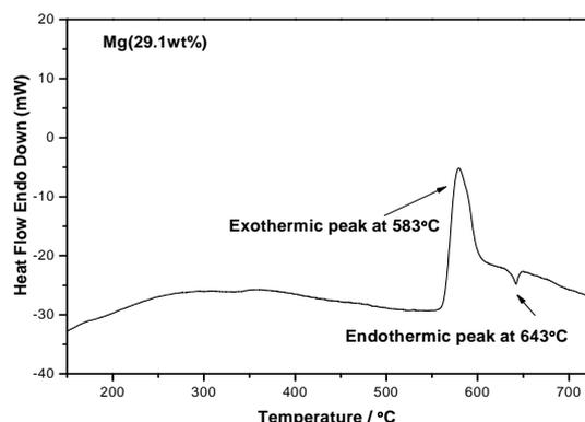
Figure 1. DTA curve of the Mg-70.9wt%Fe<sub>3</sub>O<sub>4</sub> sample
