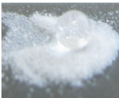
Figure 5 Photograph of water droplet on the surface of the sample
