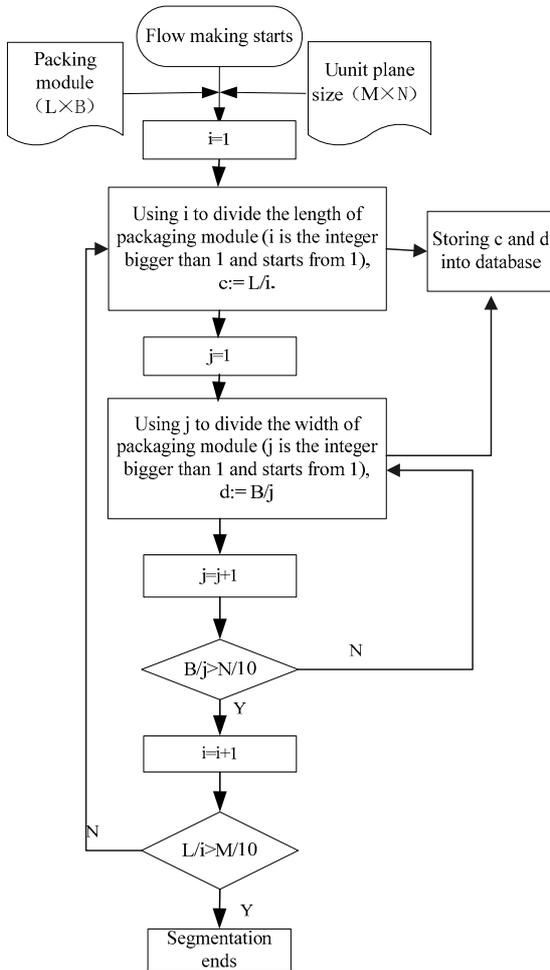
Figure 2. Flow of the process of making packaging modulus divisor dimension series.
