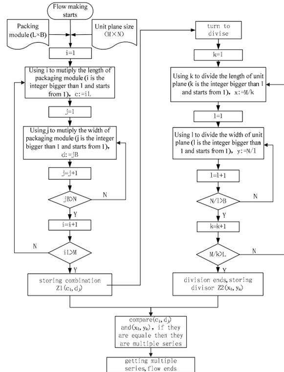
Figure 1. Flow of the process of making multiple series.
