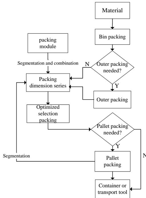
Figure 3. Sketch map of material loading process.
