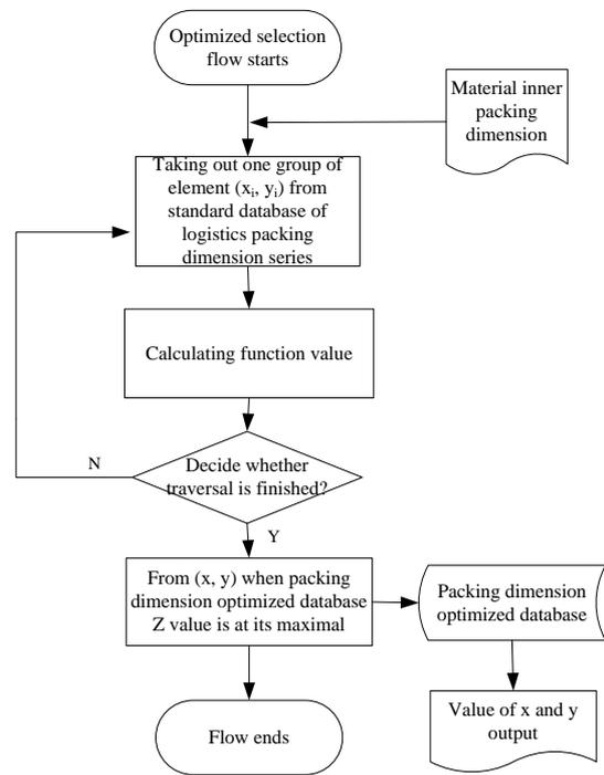
Figure 4. Process of packaging dimension choice.
