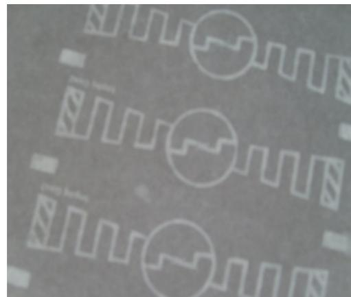
Figure 8. Patterns printed by screen printing with watermark varnish
