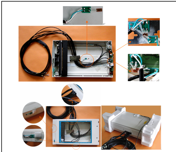
Figure 10. The location of strain gauges
