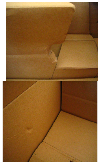
Figure 7. The breakage after the drop test at falling height of 90 cm in scheme 1
