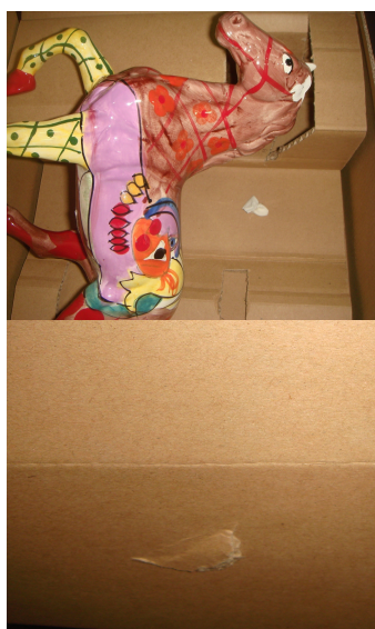
Figure 9. The breakage of C-flute at falling height of 90 cm
