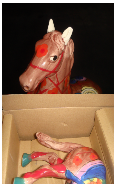
Figure 8. The breakage of B-flute at falling height of 90cm in scheme 2
