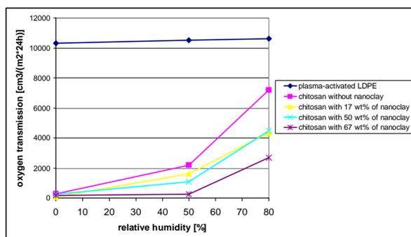
Figure 2. Oxygen transmission rates of different coatings.
