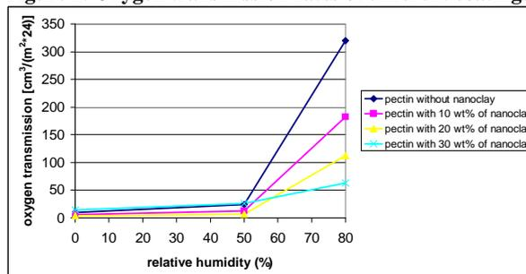
Figure 3. Oxygen transmission rates of solvent cast pectin films (100 μm) with different amounts of nanoclay.
