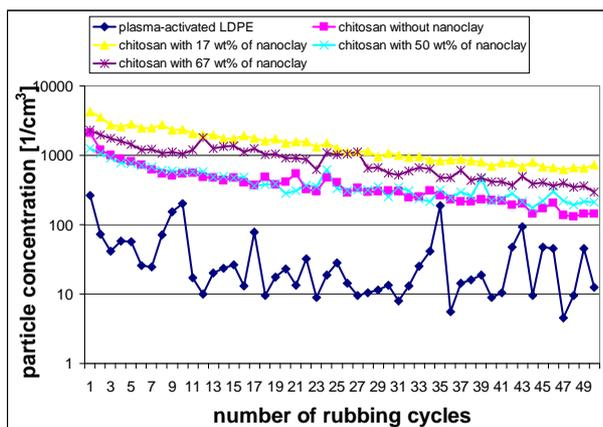
Figure 4. Particle concentration of 500 nm sized particles in air during rubbing of different coatings
