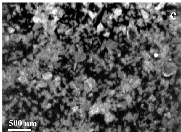
Figure 1. SEM images of (a) large undispersed nanoclay aggregates. The excerpt shows the surface structural features: lamina fine structure can be seen on the aggregate surfaces, (b) spincoated nanoclay platelets after dispersing with the ultrasonic microtip, and (c) spincoated nanoclay platelets after high pressure fluidizer treatment.
