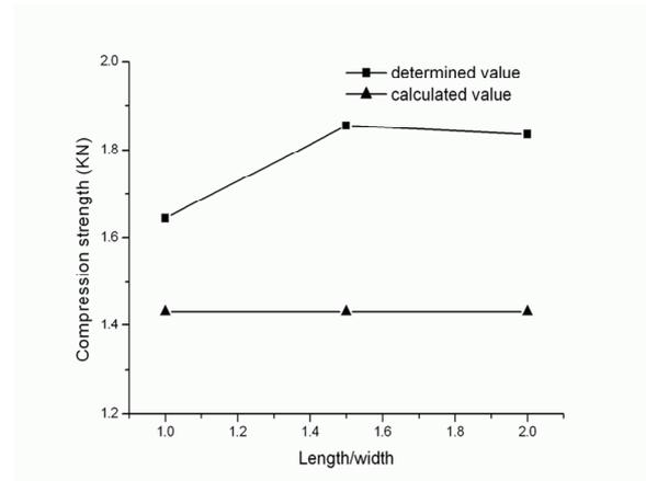
**Figure 4. Influence of base ratio on compression strength of boxes with height of 30 cm and perimeter of**
