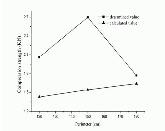
**Figure 2. Influence of perimeter on compression strength of boxes with height of 40 cm and base ratio of 1.5.**
