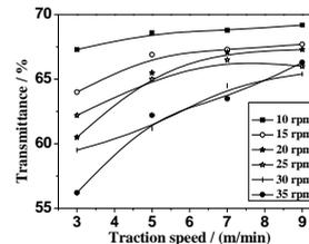
Fig.11 Influence of different film-blowing processes on the transmittance of the EVOH/SiO<sub>2</sub> composite film
