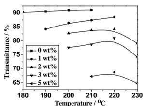
Fig.15 Influence of processing temperature on transmittance of composites
