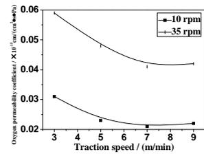
Fig.10 Influence of the traction speed on the oxygen permeability of the EVOH/SiO<sub>2</sub> composite film. (5 wt% SiO<sub>2</sub>)
