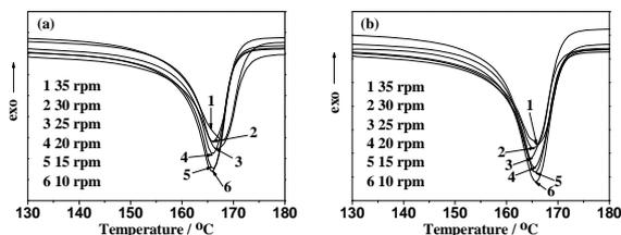
Fig.2 Influence of the extrusion speed on the melting curve of the EVOH/SiO<sub>2</sub> composite Film (traction speed: 7 m/min). (a) 0 wt% SiO<sub>2</sub>; (b) 5 wt% SiO<sub>2</sub>)
