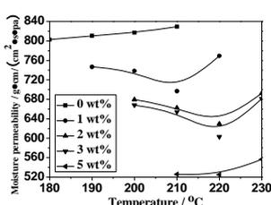
Fig.14 Influence of processing temperature on moisture permeability of composites
