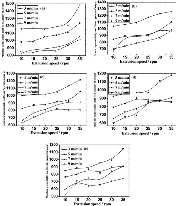
Fig.7 Influence of different film-blowing processes on the moisture permeability of EVOH/SiO<sub>2</sub> composite film. ((a) 0 wt% SiO<sub>2</sub>; (b) 1 wt% SiO<sub>2</sub>; (c) 2 wt% SiO<sub>2</sub>; (d) 3 wt% SiO<sub>2</sub>; (e) 5 wt% SiO<sub>2</sub>.)
