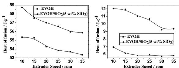
Fig.3 Influence of the extrusion speed on the fusion heat of the EVOH/SiO<sub>2</sub> composite film. (traction speed: 7 m/min)
