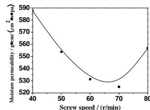
Fig.18 Influence of screw speed on moisture permeability of composites
