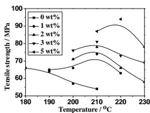
Fig.13 Influence of processing temperature on tensile strength of composites
