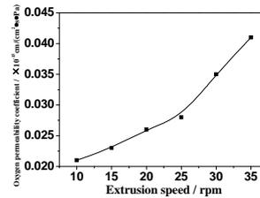
Fig.9 Influence of the extrusion rate on the oxygen permeability of the composite film (5 wt% SiO<sub>2</sub>), traction speed: 7 m/min
