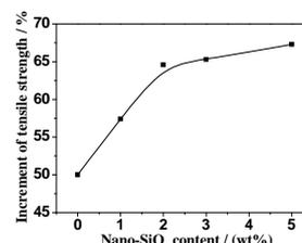
Fig.6 Influence of different amount of SiO<sub>2</sub> on the increment of tensile strength of the films
