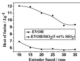
Fig.4 Influence of the extrusion speed on the differential value of fusion heat of the EVOH/SiO<sub>2</sub> composite film. (traction speed: 7 m/min)
