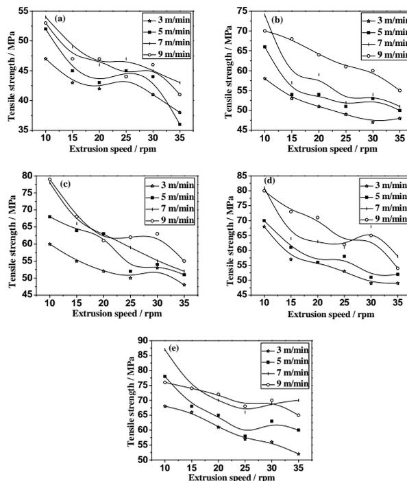
Fig.5 Influence of different film-blowing processes on the tensile strength of EVOH/SiO<sub>2</sub> composite film ((a) 0 wt% SiO<sub>2</sub>; (b) 1 wt% SiO<sub>2</sub>; (c) 2 wt% SiO<sub>2</sub>; (d) 3 wt% SiO<sub>2</sub>; (e) 5 wt% SiO<sub>2</sub>)
