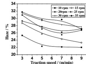
Fig.12 Influence of different film-blowing processes on the haze of the EVOH/SiO<sub>2</sub> composite film.
