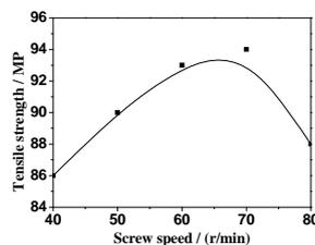
Fig.17 Influence of screw speed on tensile strength of composites
