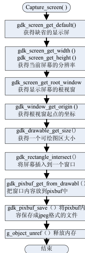
Figure 1. Flowchart: Screen capture module
