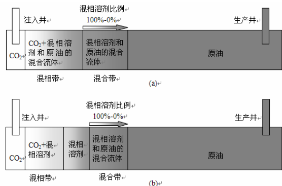
Figure1. Schematic of reducing miscibility pressure in CO 2 miscible displacement by miscible solvent method
