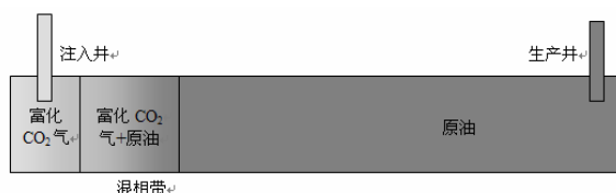
Figure 2 Schematic of reducing miscible pressure in \text{CO}_2 flooding by enriched gas miscible method
