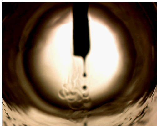
Figure5. Droplet Shape after \text{CO}_2 and oil reaches miscible
