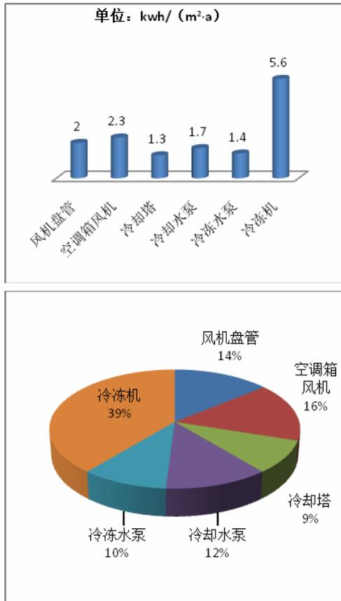
Figure 4. Some typical government office building semi-central air-conditioning system power consumption proportion [4]
