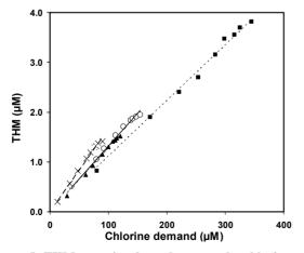
Figure 5. THM quantity dependence on the chlorine consumed in samples 1 ( $\blacksquare$ ), 2 ( $\circ$ ), 3 ( $\blacktriangle$ ) and 4 ( $\times$ ).
