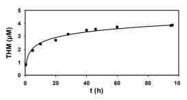
Figure 1. Dependence of the average THM quantity on the time of chlorination process.
