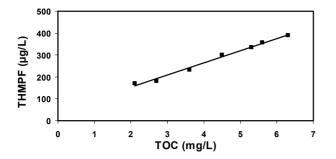
Figure 9. Correlation between the THM forming potential (THMFP) and total organic carbon concentrations (TOC).
