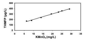
Figure 7. Correlation between the THM forming potential (THMFP) and natural organic matter concentrations (KMnO<sub>4</sub>).
