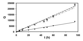
Figure 6. Formation of THM from chlorination of natural organic matter as a function of time in samples 1 ( $\blacksquare$ ), 2 ( $\circ$ ), 3 ( $\blacktriangle$ ) and 4 (×).
