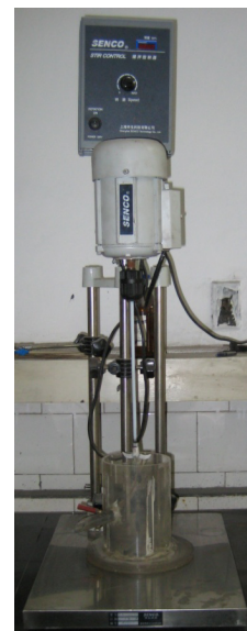
Figure1 Unit used for shear-flocculation Experiments
