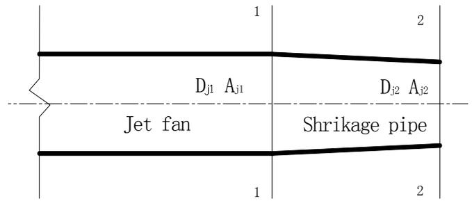
Figure 1. Install shrinkage pipe at the jet fan outlet
