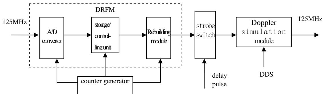
Figure 2. The Structure Chart of Frequency Storage and Signal Simulation
