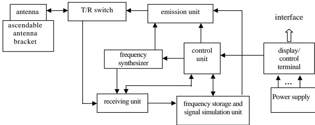
Figure 1. The Structure Chart of Active Beaconsing Equipment
