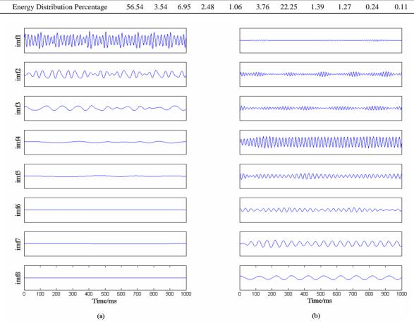
Figure 7. (a) IMFs obtained by EMD with the original vibration signal; (b) IMFs obtained by EMD with the reconstructed signal by WPT and correlation degree threshold screening
