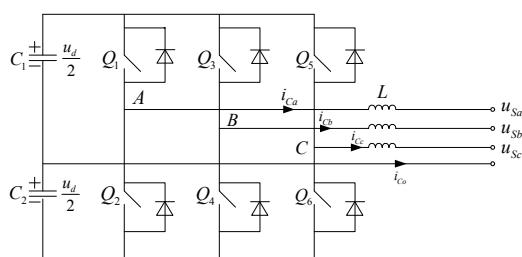
Figure 2. APF circuit structure of aircraft electricity grid
