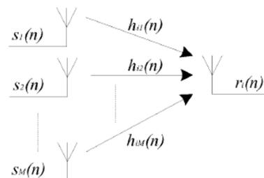
**Figure 1. Signal transmission of MIMO-OFDM communication system**
