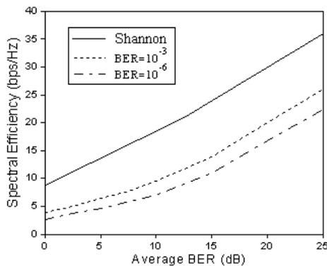
Figure 4. The spectral efficiency of adaptive MIMO-OFDM communication system in the case of the constellation size unlimited
