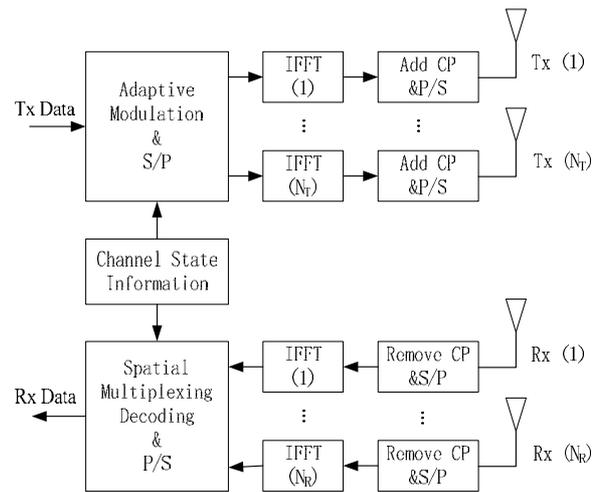
Figure 3. Adaptive MIMO-OFDM communication system model
