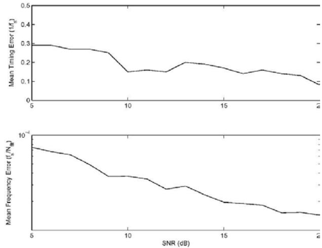
Figure 2. Synchronizer performance curves at different receiving SNR
