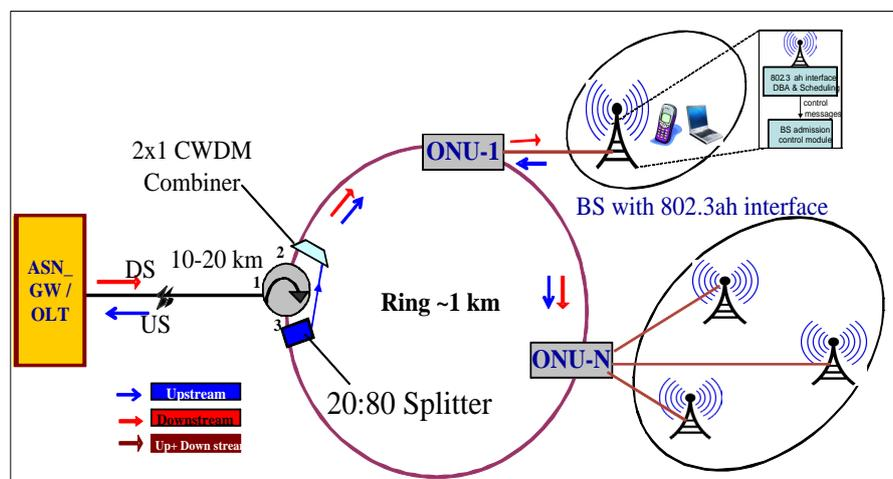
Figure 1. EPON-based RAN architecture.
