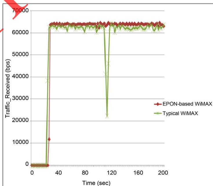
**Figure 10.** Traffic throughput during MS handoff.
