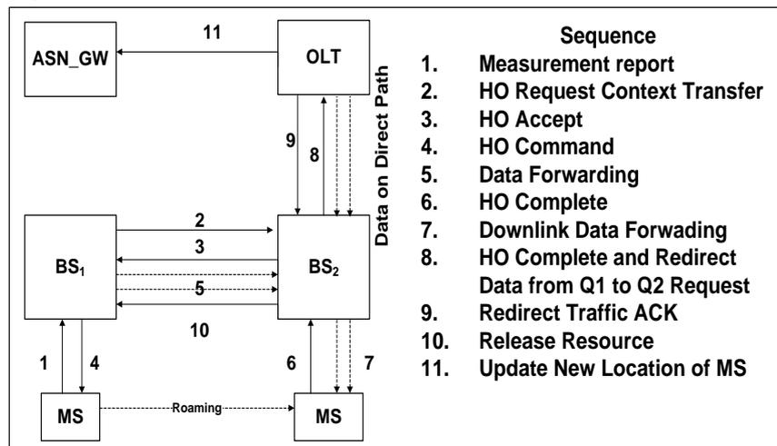
**Figure 4.** Sequence of the intra-OLT HO procedure between the source and the target.
