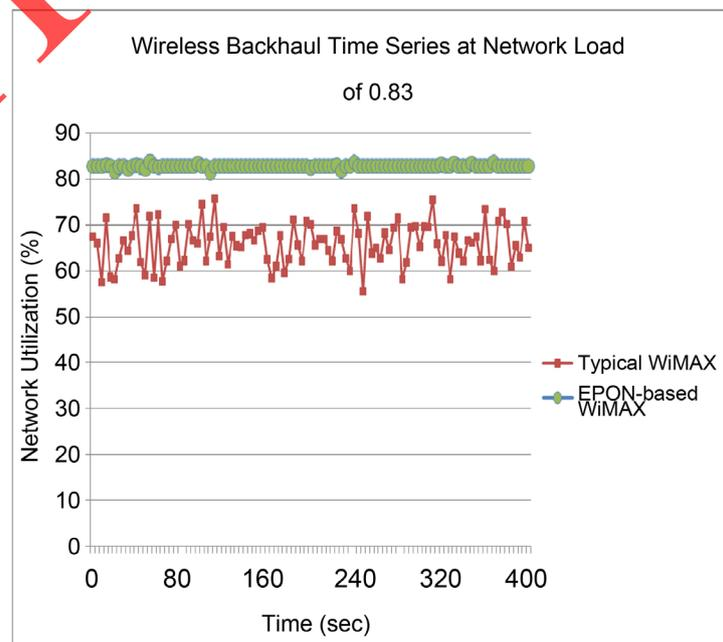
Figure 5. Uplink utilization time series at network load = 0.83.
