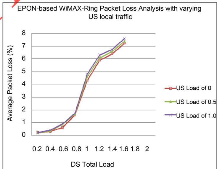
**Figure 9.** Average packet loss of DS traffic as a function of US local load in EPON-based WiMAX ring network.
