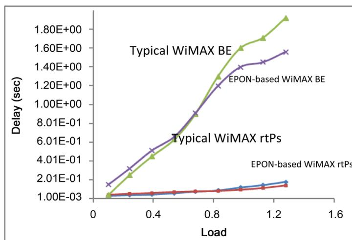
Figure 7. Average network ETE delay for rtPs and BE traffic.
