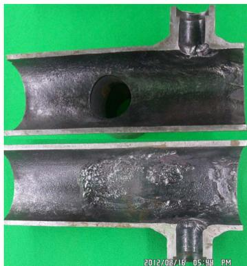
**Figure 2.** Damaged surface by LDIE.
