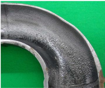
**Figure 1.** Damaged surface by FAC.
