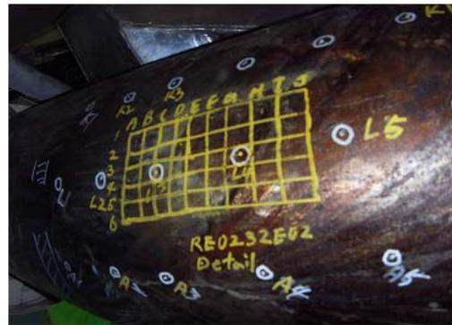
Figure 7. Grid layout for a detailed UT examination.
