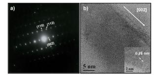
Figure 3. (a) Electron diffraction pattern from a single nanorod. (b) HRTEM image of a nanorod. The nanorod grows along [002] direction.
