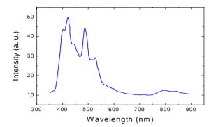
Figure 4. Spectrum of photoluminescence of the ZnO nanorods under 358 nm excitation.
