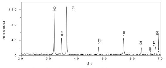
Figure 1. Diffraction pattern of the nanorods ZnO nanostructures.
