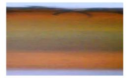
Figure 5. Gross-section of a CdS/PVA film nanocomposite of 15 cycles (film is 350 µm in thickness).
