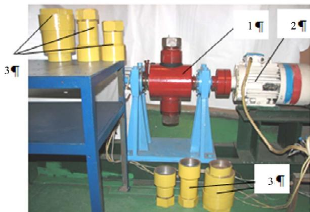
**Figure 2.** Overall view of a centrifugal SHS facility: (1) rotor; (2) electric motor, (3) changeable chamber with refractory mould.
