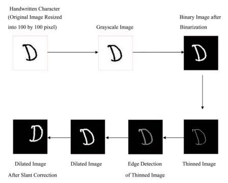
Figure 4. Results of preprocessing steps applying on a handwritten character.
