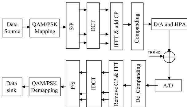
**Figure 1.** OFDM system block with DCT-companding.
