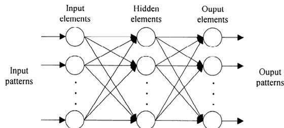
**Figure 1. Architecture of a three-layer BP network.**
