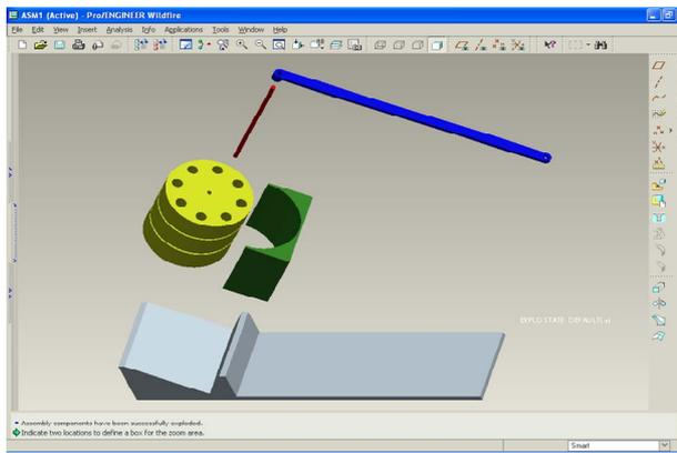
Figure 7. The motor assembly (exploded view).
