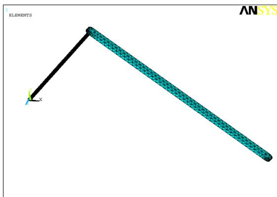
Figure 10. Shaft and crank sub assembly (FE model).
