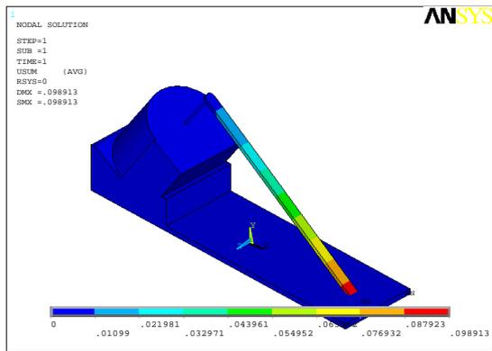
Figure 9. Deformation due to gravity.
