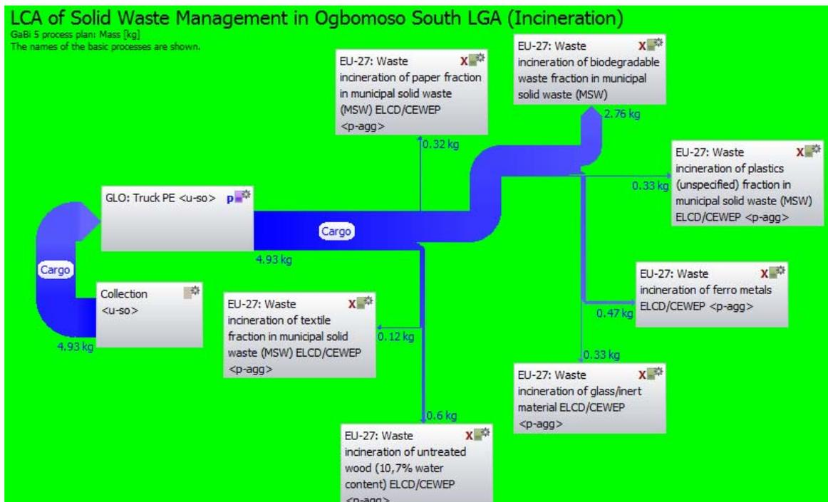
Figure 5. LCA scenario/model two of waste management developed using GaBi<sub>5</sub> software.
