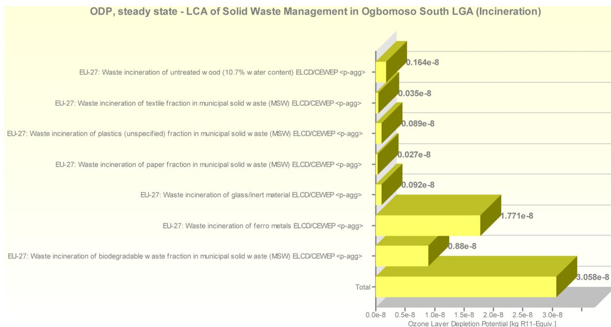
Figure 21. LCIA for incineration (CML-ODP).
