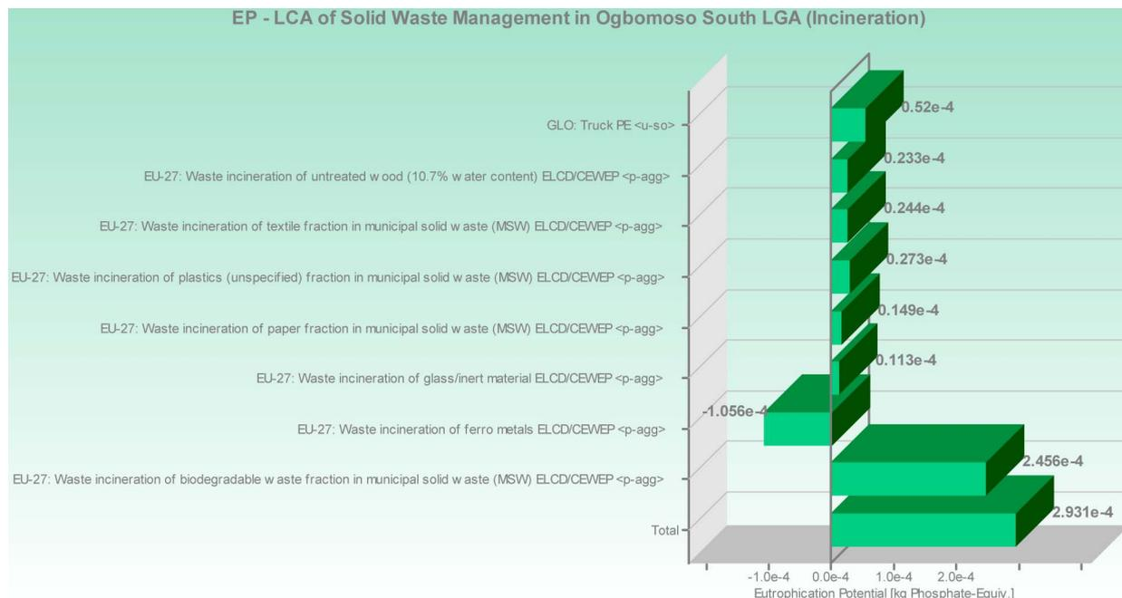
Figure 20. LCIA for incineration (CML-EP).
