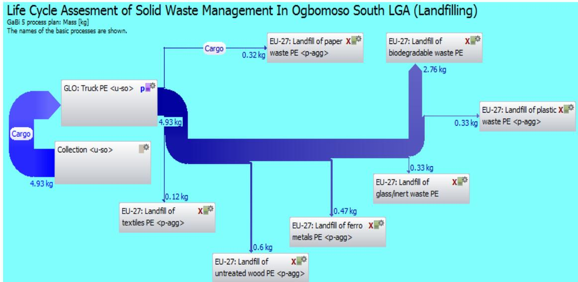
Figure 4. LCA scenario/model one of waste management developed using GaBi<sub>5</sub> software.
